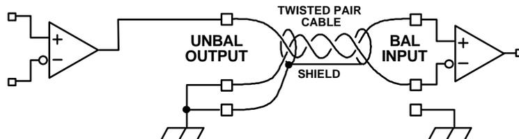
The triangles symbolize electronic amplifiers inside equipment and the larger squares symbolize connections to exterior wiring. Notice that the output circuit is unbalanced, even though it has three terminals, and the input remains balanced, even though only two terminals are used.
