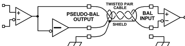
This schematic shows a polarity-flip type output properly wired to a balanced input, such as those of the DFP-D3000. Neither output polarity will be shorted to ground and equipment grounds remain isolated. Signal level is unaffected.
