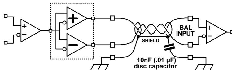
A small disc ceramic capacitor is inserted into the connection between the shield and ground at one end only.
