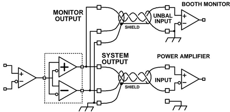
Notice that the unbalanced input of the booth monitor effectively unbalances the output of the DFP-D3000, as it connects the – or “cold” out-of-phase side to the booth monitor’s ground. Nevertheless, if the wiring is done as illustrated the power amplifiers will suffer no hum problems. Chassis grounds of all three pieces of equipment will not be connected together by the wiring, and no component of the audio signal flows in shields.
