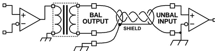
Notice that this connection still provides electrical isolation between the chassis grounds of the two pieces of equipment, providing that the cable shield is managed as shown. Here is the equivalent electronically balanced version:
