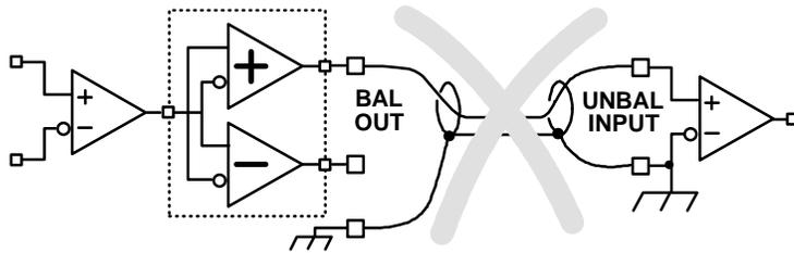
*Do not make your connections in this manner!* This connection results in an undefined signal that could result in problems with stability, level, headroom, and frequency response. It also connects the grounds of the two pieces of equipment together using the return path of the audio signal, which could result in hum. Connecting the – phase of the balanced output to its own ground terminal is a poor compromise which should only be used as a last resort.
